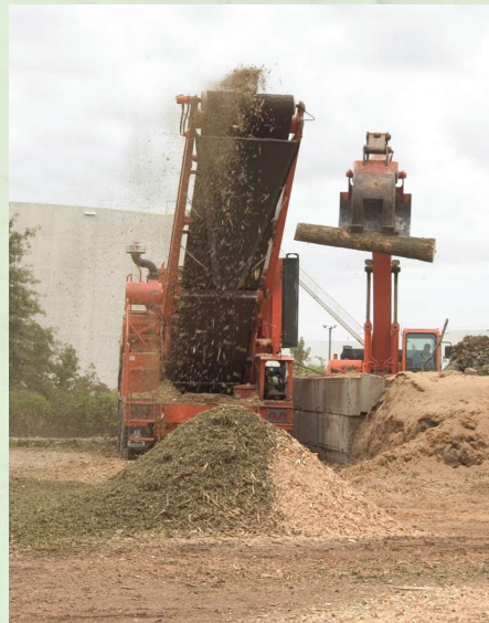
Figure 15 —In New Jersey, woody debris from ALB Program activities is chipped prior to incineration at a local cogeneration plant.
